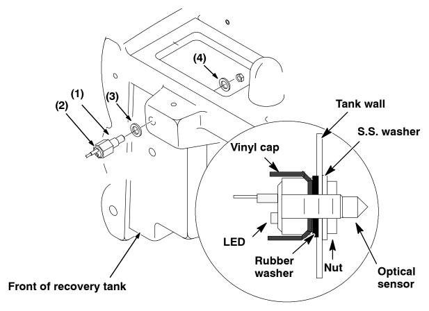
FIG. 2 Switch Installation
