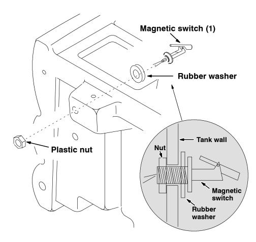
FIG. 1 Magnetic Switch Removal
